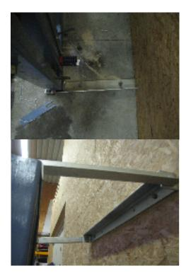
The wall mounting can easily be lifted of the door and folded straight down if the door needs to be moved to another location.
