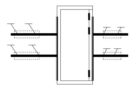
Welding the tactical training door into a container must be done with caution. The heat from welding may cause the metal to twist or bend. We recommend that you only weld at some points on the frame and not along the entire side.
